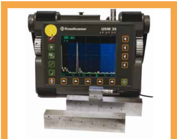
A shear wave probe on carbon steel block
